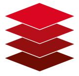
Protection Film (10 μm) Non Yellowing TPU (150 μm) Adhesive (35 μm) Release Liner (75 μm)
